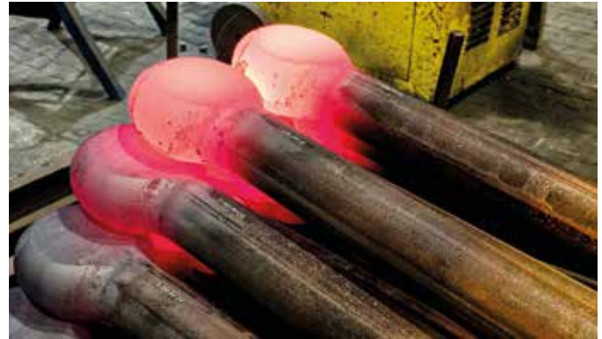
Zero-waste forging process: eyes are upset forged
