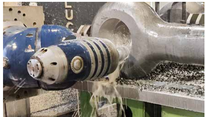
Shackles and pins CNC machined
