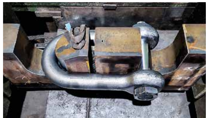
Proof testing (2 x WLL) using quick release system
